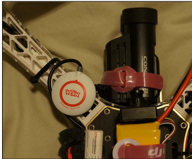
THIS QUADCOPTER IS FLOWN IN A LOCATION THAT HAS 10 DEGREES EAST (POSITIVE) DECLINATION. NOTICE HOW THE GPS IS ROTATED RIGHT 10 DEGREES
